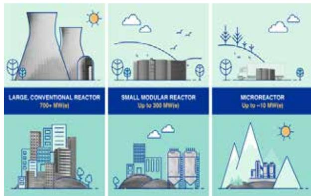
Small modular reactors (SMRs) have a power capacity of up to 300 MW(e) per unit. Many SMRs, which can be factory-assembled and transported to a location for installation, are envisioned for markets such as industrial applications or remote areas with limited grid capacity.
