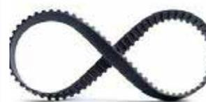
valves open and close once every other turn of the crankshaft. The timing belt performs this very important job. It has custom teeth to turn the camshaft(s) in sync with the crankshaft and is specifically designed for each particular engine. In some
